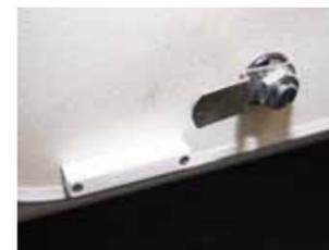
Simple systems are sometimes the best. Before work commences every locker or door that has to be protected gets a bit of black insulating tape. After it is wired up, the tape is removed. Easy!
