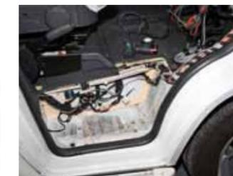
Some competitors will just tuck wiring under carpets, but Vanbitz removes the step moulding to ensure a neat job
