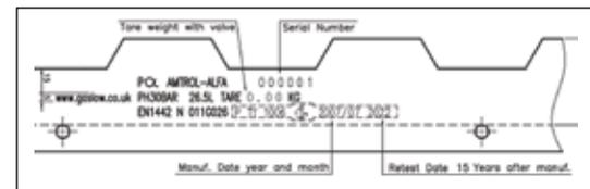
Your cylinders are manufactured to European Standard EN1442 and each one has its own unique certificate and identification stamped into the bottom foot shroud of the cylinder.
