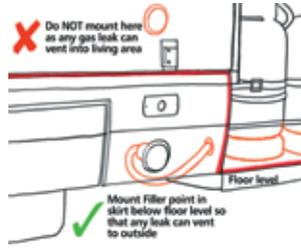
Fit in the skirt of the vehicle, below the floor level as any escaping gas can then vent freely to the atmosphere
