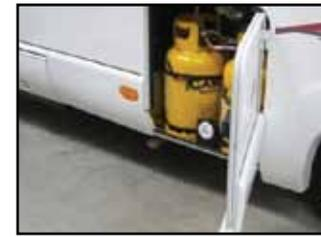
Installation using Mounting Bracket with a 0.6metre hose and right angle adaptor
