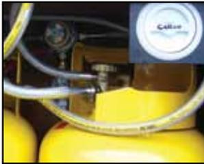
Use the Filling Point Mounting Bracket in the cylinder compartment - either between the cylinders or top mounted.
