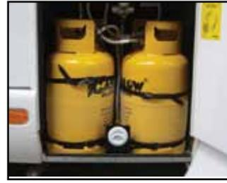
Installation using a bracket in the cylinder compartment should use a 0.6 metre hose
