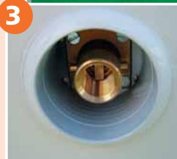
**4** Line up the filler nozzle to the two lugs and then give it a third of a turn clockwise to seal it securely.
