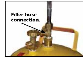
Install cylinder No.2 by connecting the filler hose to the horizontal inlet and the 2nd cylinder connection hose to the top inlet.
