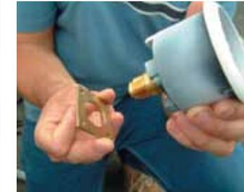
Install the Brass Filler head into the bracket using the 4 screws and bracket provided
